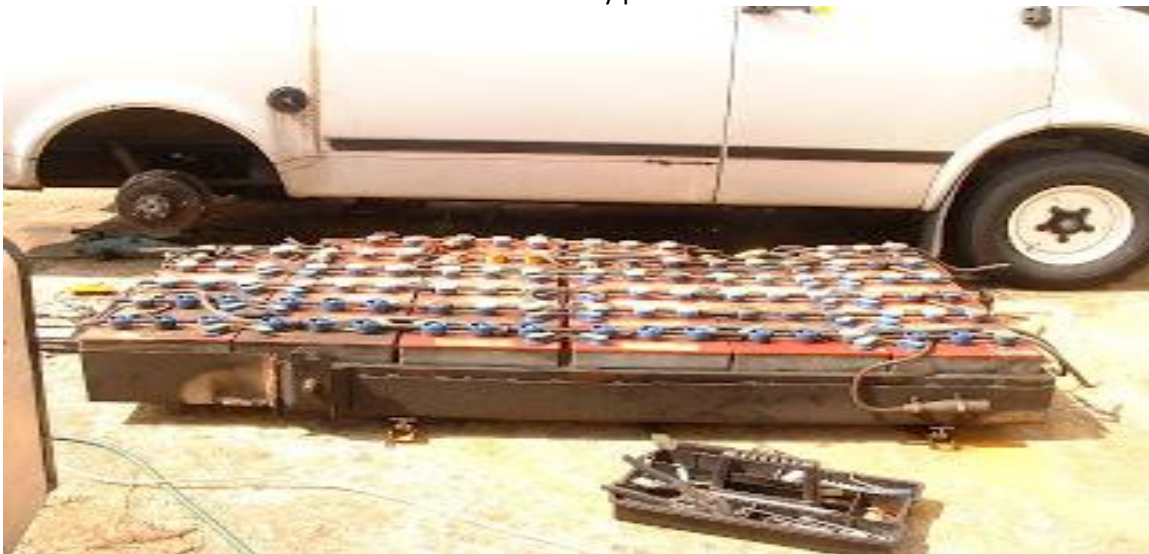
“View of the battery pack all 1Ton of it”
